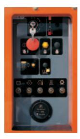
**Gound Console.** Accessible location, high-contrast colors, and large graphic symbols facilitate console operation. The manual descent system can be operated from the chassis to lower the platform in an emergency. An optional status indicator light panel provides information on alternator, engine oil pressure, engine coolant temperature, and hydraulic oil filters.
